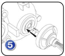
INSERT LED BULB WITH DUST BOOT INTO MOUNTING PLATE.
