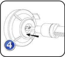
INSERT LED BULB INTO RUBBER DUST BOOT.
