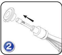
REMOVE MOUNTING PLATE FROM LED BULB
