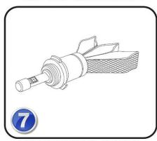
SPREAD HEATSINKS AND PLUG INTO WIRING CONNECTOR
