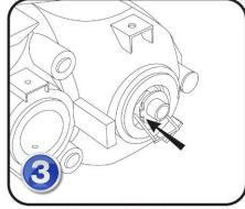
PLACE MOUNTING PLATE IN LIGHT FIXTURE AND FASTEN SPRING CLIP
