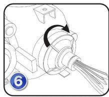
ROTATE LED BULB AND BOOT TO LOCK INTO PLACE.
