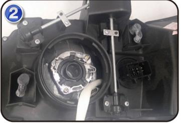
REMOVE THE MOUNTING PLATE FROM THE LED BULB AND INSTALL IT IN THE LIGHT HOUSING.
