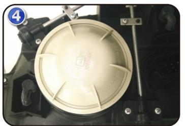
REPLACE THE DUST COVER (IF EQUIPPED) AND TEST THE HEADLIGHT.
