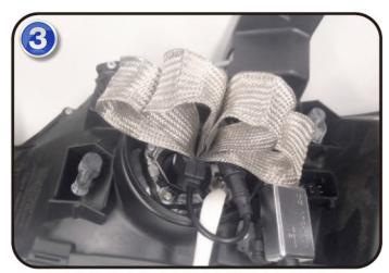
INSTALL THE BULB AND CONNECT TO POWER. SPREAD HEATSINKS AS SHOWN.
