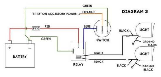
IF AN ACCESSORY SWITCH BLOCK (BBP# 13-207) OR A MASTER CYLINDER SWITCH BLOCK (BBP# 52-605) ARE INSTALLED, OMIT THE ROCKER SWITCH AND CONNECT THE BLUE WIRE ON THE RELAY TO AN OPEN SWITCH ON THE SWITCH BLOCK.
