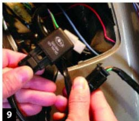
9 Plug the four-pin switch connector into the relay harness, and plug the relay harness into the motorcycle accessory four-pin connector. The kit also comes with a jumper plug which can be used in place of the relay which makes the lights function only with the switch.
