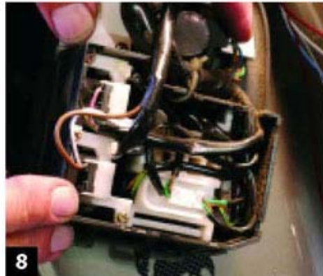
8 Moving to the left side fairing, remove the trim, control panel, and switch cover located on the back of the control panel. Remove the switch hole cover and install the new switch in it's place.
