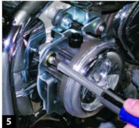
5 Fit the lamp bracket onto the mounting bracket and attach it with the short flange and longer Phillips head screws.
