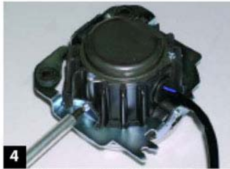
4 Install the fog lamp to the right bracket with three small Phillips head screws.
