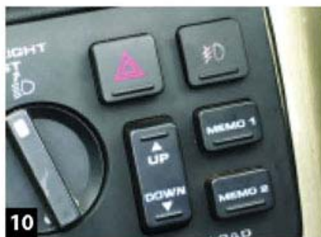
10 After testing the lights, reinstall the control panel. The new switch looks stock, and is illuminated whether the fog lights are on or off.
